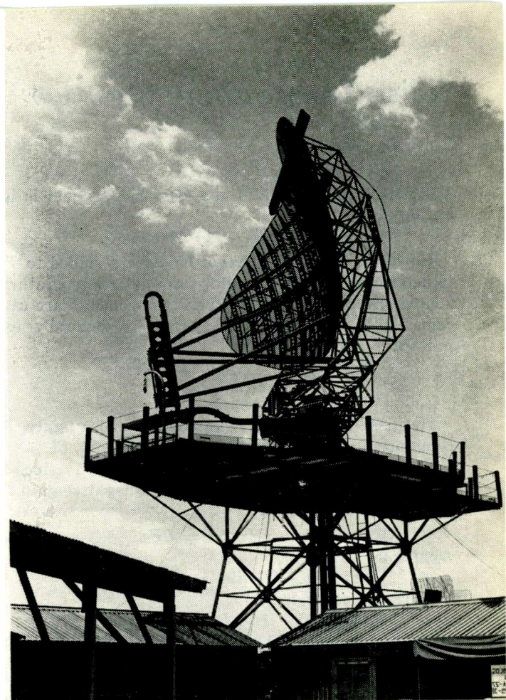
Long range search radar antenna made by Bendix for the AIR Force.
