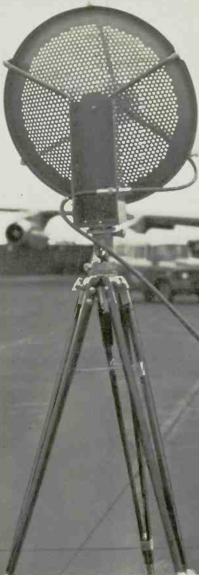
Polarad Model SA-84W being used to make pulse analysis of radar aboard a Pan American Boeing 707, Jet Clipper®
