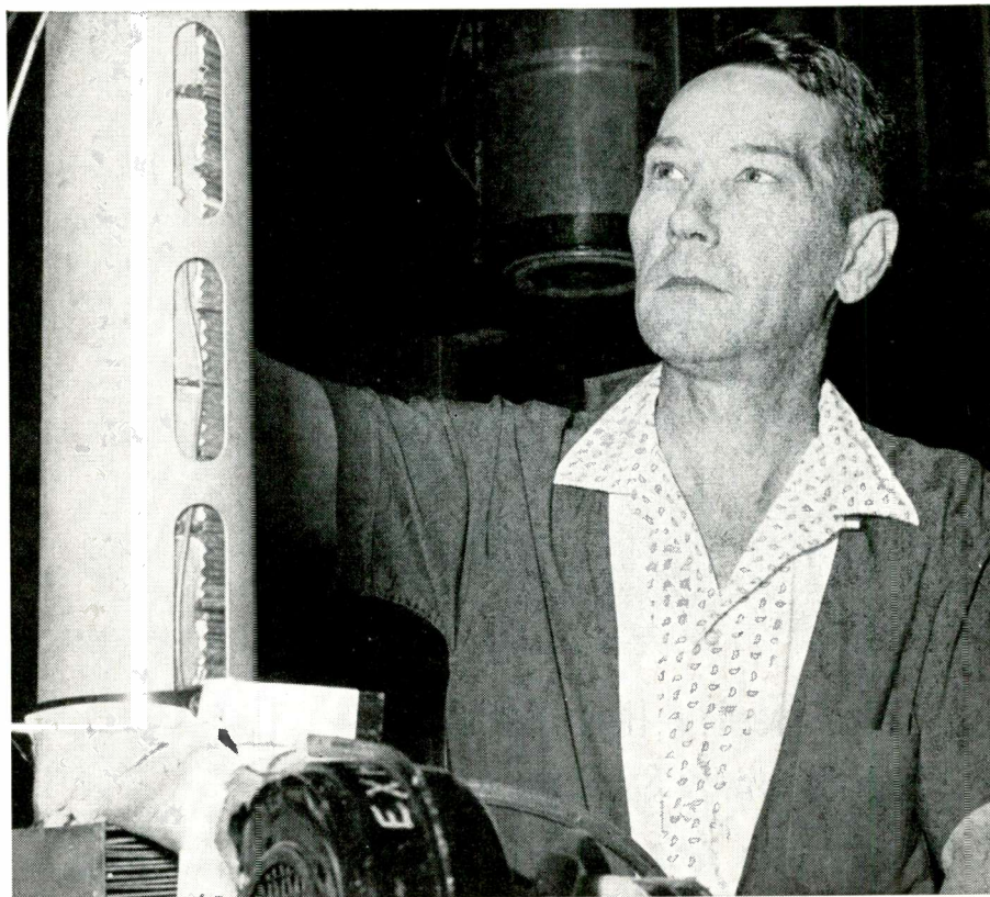
FACTORY ALIGNMENT of a Sperry TWT within its focusing solenoid greatly simplifies field maintenance. Once this operation has been performed by a skilled Sperry technician, the assembly is self-aligning.
