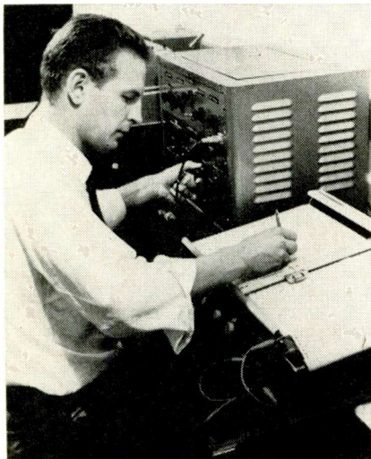
D. Bickler, solar measurements specialist, takes readings from a monochrometer and verifies that light output from solar simulator developed by Hoffman Electronics Corp. has the same qualities as actual sunlight in outer space.
